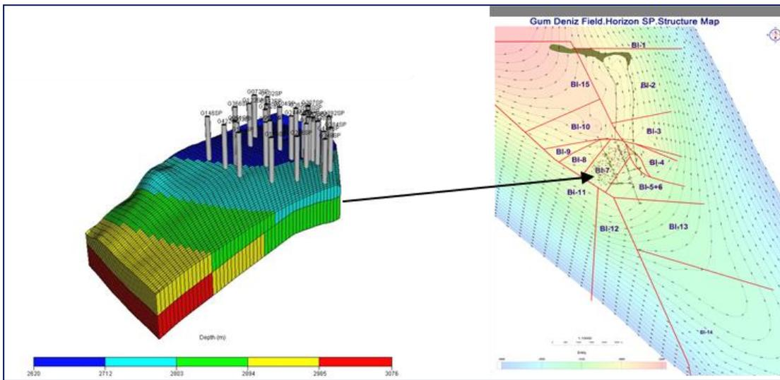
Figure 2. SP structure map with blocks and reservoir model with production wells
