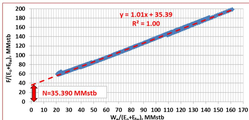
Figure 1. Material balance plot for N with  $E_{fw}$  term
