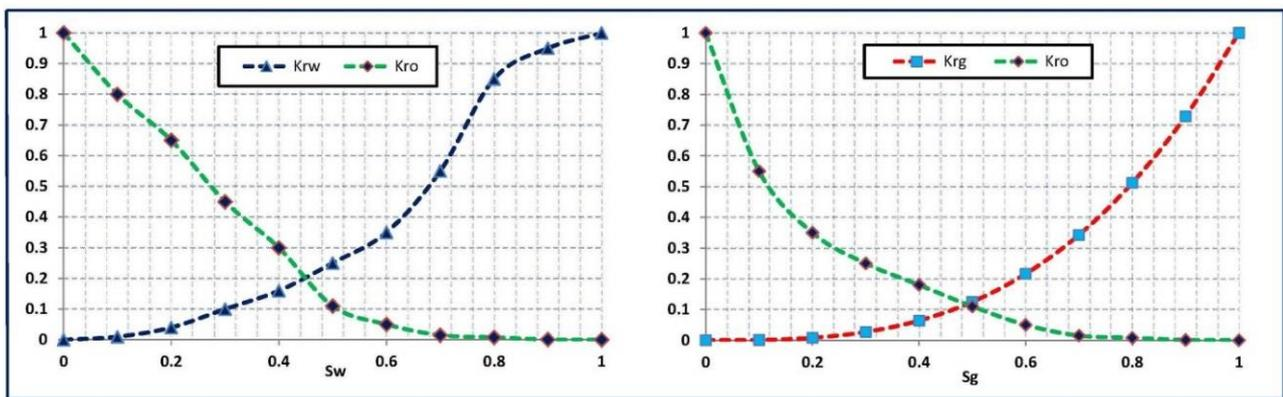
Figure 3. Oil-water & gas-oil relative permeability
