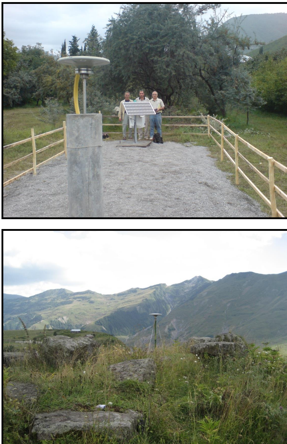
Figure 2. A – GPS continuously recording station located in Sheki, Azerbaijan. B – GPS survey site in the Greater Caucasus. The antenna is precisely located above the mark that is cemented into the bedrock
