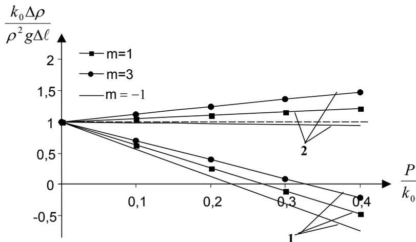
Fig. 2. Density changes of granite and quartz at increasing pressure according to non-classical linearization theory
