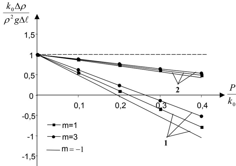
Fig. 1. Qualitative results about the pressure change impact on moveout density of organic glass.
