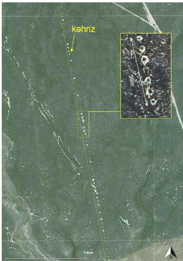
Fig. 2. Preliminary results of the qanat (kehriz) discovery in the Gobustan area (I). The yellow-dashed line follows the qanat shaft line, which may be traced up to several kilometers from the inlet. Satellite images are taken in May 2009 (main image) and October 2023 (enlarged area). The distance between shafts is 4-5 m
