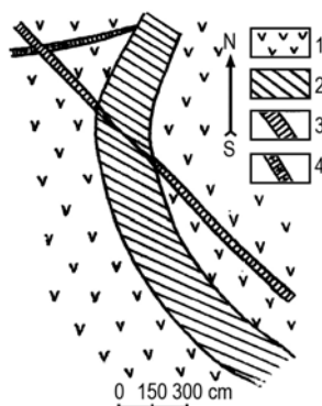
Fig. 9. Age relationship between a diorite porphyrite dike and two mineralized fractures of different directions. Gazikhanli area. 1 – porphyrites; 2 – dike; 3 – gold-bearing zone in NW direction; 4 – galenite-bearing zone in NE direction
